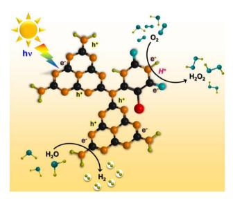
Scheme 1 Schematic illustration of photocatalytic  $H_2O_2$  production and hydrogen generation (the black, orange, blue, green, and red spheres represent C, N, O, H, and halogen ions).
