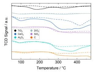
Fig. 2 TCD-signal during CO<sub>2</sub>-TPD experiments, for pure support (dashed lines) and Ru/support (solid lines).
