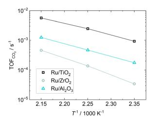
Fig. 7 Arrhenius-plot based on the TOF from CO<sub>2</sub> consumption rate.
