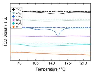
Fig. 1 TCD-signal during H<sub>2</sub> TPR measurements, for pure support (dashed lines) and Ru/support (solid lines).
