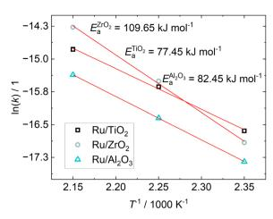
Fig. 6 Arrhenius-plot from the kinetic constant obtained from parameter fitting *via* eqn (8) and the resulting apparent activation energy for different catalysts.
