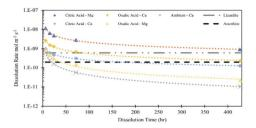
Fig. 14 Measured dissolution rates based on release of Mg and Ca in 0.5 M citric and oxalic acid solutions. Compared to measured Ca release rate and steady state anorthite dissolution, both at ambient temperature/pressure and pH =  $4.19.^{10,31}$
