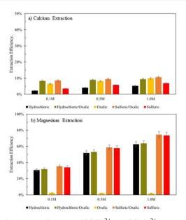
Fig. 12 Extraction efficiency of (a) Ca<sup>2+</sup> and (b) Mg<sup>2+</sup> in mineral acid series dissolution, compared to single acid dissolution. Data organized by the solution concentration step of the series. Naming convention refers to the order of the acid(s) used.
