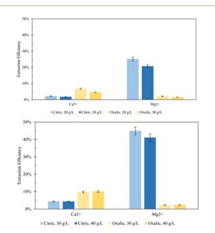
**Fig. 6** Effect of solid/liquid ratio on calcium and magnesium extraction in 0.5 M citric and oxalic acid solutions dissolving for (top) 18 hours and (bottom) 72 hours. Percentage differences are displayed above each set of bars.
