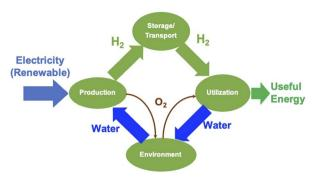
Fig. 4 Splitting of water ( $H_2O$ ) using renewable electricity is a net-zero emission process and is also circular in nature, becoming completely sustainable. This is because the product of  $H_2$  combustion will produce  $H_2O$ , which can be reused if collected at the source and recovered completely. This process can be least harmful both environmentally and ecologically.
