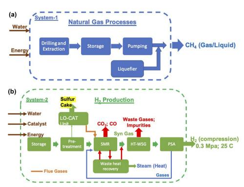
Fig. 8 System boundary of the SMR process for life cycle assessment can be split into two distinct stages. Stage 1, (a), concerns natural gas mining, extraction and transport to the final usage site, while Stage 2, (b), is exclusively concerned with steam methane reforming of natural gas to produce  $H_2$ , which can be compressed for transport. The  $H_2$  produced will be of 99.9% purity and in gaseous form. Some life cycle assessments consider only Stage 2, while some consider both stages.
