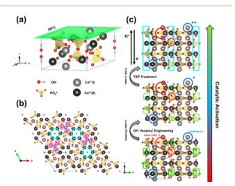
Scheme 1 Structure of HAp as a catalyst. (a) HAp unit cell  $P6_3/m$ . (b) (001) crystallographic plane observed from the c-axis direction. The OH $^-$  channels and the Ca(ı) 6-fold coordination are highlighted. (c) Structural changes and lattice refinement strategies adopted to achieve the catalytic activation of HAp.
