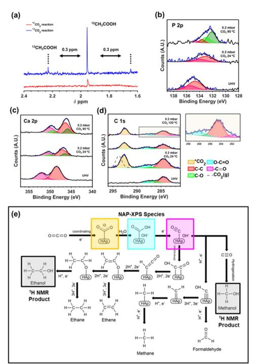
Fig. 4 (a) Isotope-labeling experiments. High resolution NAP-XPS studies using  $^{12}CO_2$  of the P 2p (b), Ca 2p (c) and C 1s (d). (e) Fixation mechanism derived from  $^1H$  NMR and NAP XPS results.
