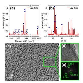
Fig. 1 (a) Raman spectrum, (b) XRD diffractogram, (c) SEM and (d) HRTEM micrographs, and (e) fast Fourier transform of the HRTEM micrograph for upp-HAp. In (a) the characteristic HAp ( $\nu_1-\nu_5$ ) and brushite (diamonds) Raman vibrational modes are displayed. In (b), the characteristic HAp (spots) and brushite (diamonds) reflections are indicated.
