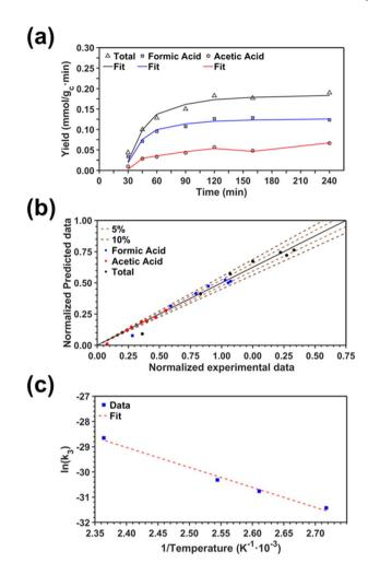
Fig. 5 Comparison between the experimental data and the fitting model: (a) fitting of the different experimental yields obtained from the kinetic models proposed; (b) parity plot; and (c) linearization of the Arrhenius expression.
