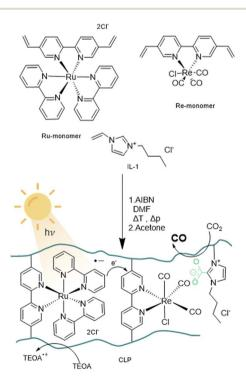
Fig. 1 Schematic representation of monomers used for the radical polymerisation of crosslinked polymers (CLP) with AIBN (azobisisobutyronitrile) towards a polymer framework for photocatalytic CO<sub>2</sub> reduction.
