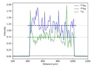
Fig. 4 LA-ICP-MS line scan for <sup>101</sup>Ru (red) and <sup>185</sup>Re (green) normalized to the <sup>13</sup>C isotope (black, dotted). Average intensity for each isotope is depicted as dotted line.
