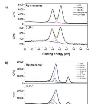
Fig. 3 Detailed XPS scans of CLP-1 and monomers. Re 4f (a) and C 1s together with Ru 3d<sub>5/2</sub> (b)
