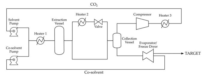
Fig. 5 Scheme of an industrial SCF extractor (adapted from ref. 64 with permission from Elsevier).
