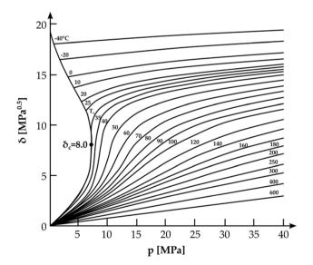
Fig. 2 Isothermal curves of the Hildebrand solubility parameter for CO<sub>2</sub> as a function of pressure (adapted from ref. 54 with permission of Elsevier).
