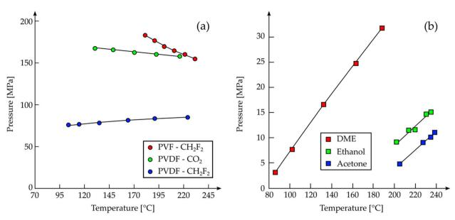
Fig. 7 (a) Cloud points of PVF in  $CH_2F_2$  (red) and PVDF in  $CO_2$  (green) and in  $CH_2F_2$  (blue); (b) cloud points of PVDF in  $CO_2$  with dimethyl ether, DME (red), ethanol (green) and acetone (blue) as co-solvents. All graphics adapted with permission of J. S. Lim and M. A. McHugh, *J. Phys. Chem. B*, 1999, **103**, 2818. Copyright (1999) American Chemical Society.
