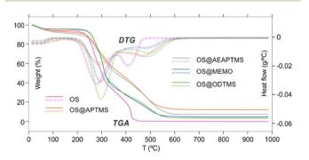
Fig. 2 TGA and DTG curves for native OS and functionalized OS@silanes.
