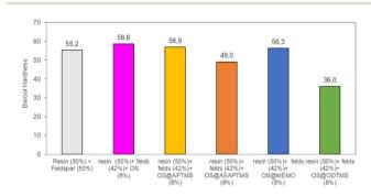
Fig. 5 Barcol Hardness measurements for the different composites obtained. All the measurements were performed in triplicate (Table S7†) with a constant conductivity of 700  $\mu$ S cm<sup>-1</sup>.
