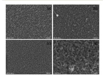
Fig. 3 SEM images of various samples grown at (a) 800  $^{\circ}$ C on silicon (b) 800  $^{\circ}$ C on quartz (c) and (d) 500  $^{\circ}$ C on quartz.
