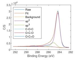
(b) Graphene on silicon substrate
