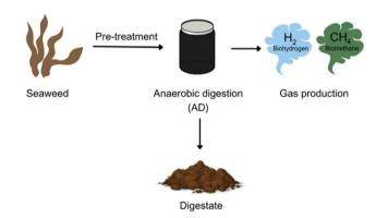
Fig. 2 Simple scheme to represent biohydrogen and biomethane production from seaweed (figure made using https://www.canva.com).
