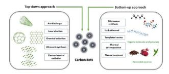
Fig. 2 Synthesis methods of CQDs and their classification.
