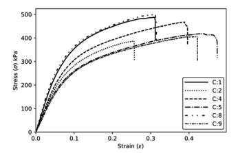
Fig. 9 Typical tensile stress-strain curves
