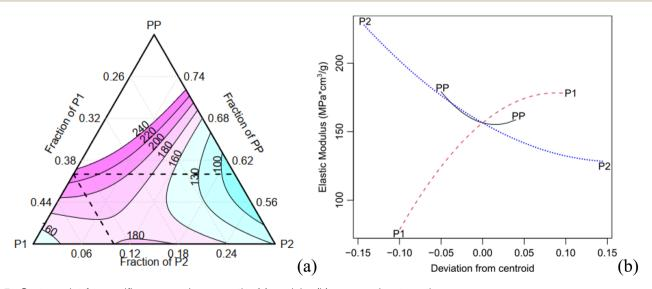
Fig. 7 Contour plot for specific compressive properties (a) modulus (b) compressive strength.
