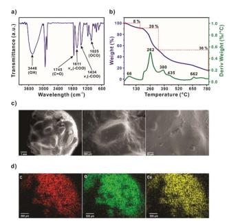
Fig. 1 (a) FT-IR spectra; (b) TGA-DTG analysis; (c) SEM micrographs; and (d) mapping of SCG\_ALG.
