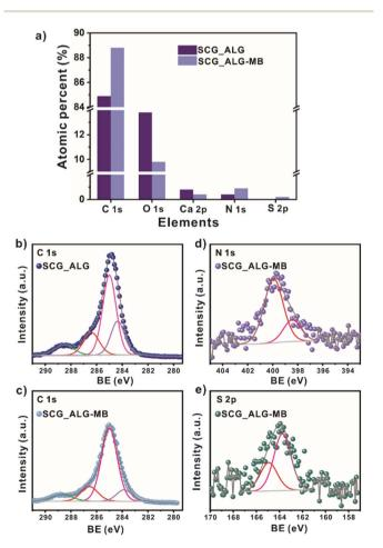
Fig. 5 (a) Atomic percent of the elements in the SCG\_ALG adsorbent before and after MB adsorption, XPS high-resolution spectra of (b) C 1s before adsorption, (c) C 1s, (d) N 1s, (e) S 2p after MB adsorption.
