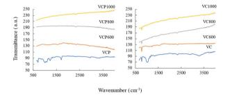
Fig. 3 FT-IR spectra of VCPs and VCs.
