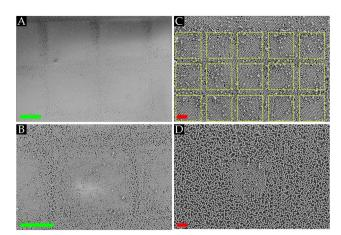
Fig. 5 SEM images of 3 μm PMMA spherical particles on the glass host substrates with (A) and (B) 200 μm CF<sub>x</sub> confined squares and spacing of 50  $\mu$ m, (C) 50  $\mu$ m CF $_x$  confined squares (indicated with dashed lines) and spacing of 10 μm, and (D) 50 μm CF<sub>x</sub> confined squares and spacing of 500 μm. Scale bar: 100 μm (green); 20 μm (red).
