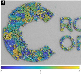
Fig. 6 (A) SEM images of 3 μm PMMA spherical particles on a CF<sub>ν</sub> pattern (shaped in the logo of the RSC) with SiO<sub>2</sub> as the host substrate, scale bar: 100 μm. (B) Same image as in (A) but now with the grain distribution highlighted. The color bar indicates the rotational orientation of the grains. A few of the excess particles remaining on the uncoated areas were removed by blowing pressurized air (4 bar) along the substrate.
