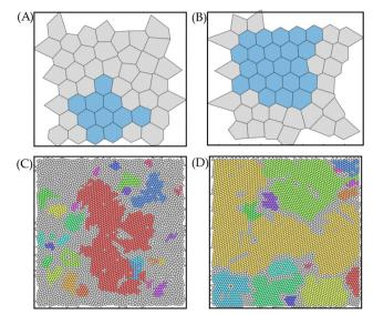
**Fig. 3** A single crystal structure identified comprising 3 μm PMMA microspheres on a CF<sub>x</sub> pattern of 25  $\times$  25 μm² on (A) glass and (B) SiO<sub>2</sub> as a host substrate. Multiple identified crystals (each coloured differently) comprising 3 μm PMMA microspheres on a CF<sub>x</sub> pattern of 200  $\times$  200 μm² on (C) glass and (D) SiO<sub>2</sub> as a host substrate.
