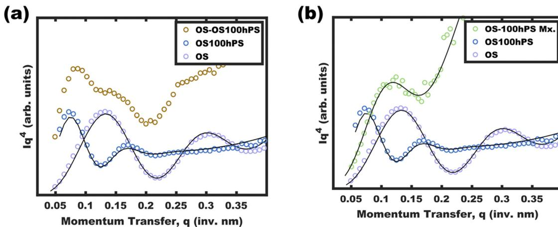
Fig. 5 SAXS data and best-fits for **OS** and **OS-100hPS** micelle stocks measured both separately and after combination in pure EtOH to yield a bimodal distribution (a). The mixture was then measured again after the addition of 30 vol% DCM with stirring for 1.5 h to yield a new equilibrated size distribution (b). Values are presented in  $Iq^4$  vs.  $q$  coordinate spaces to highlight small changes in micelle form factor oscillations.
