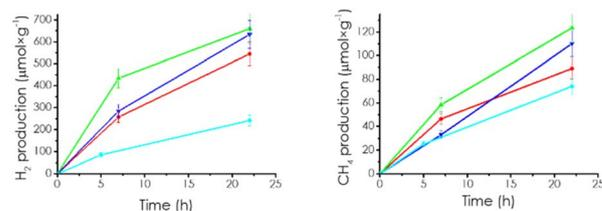
Fig. 3 Gas evolution for the samples mpC (cyan), CD-08/mpC (red), CD-1/mpC (green), CD-12/mpC (blue). Reaction conditions: acetonitrile 12 mL, H<sub>2</sub>O 4 mL, triethanol amine 4 mL, CD-*x*/mpC at 0.5 mg mL<sup>-1</sup>, irradiation through quartz with the full output of a 300 W Xe lamp.
