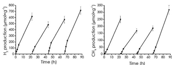
Fig. 5 Temporal hydrogen and methane evolution in the photocatalytic irradiation of CD-1/mpC in four consecutive uses. Reaction conditions: acetonitrile 12 mL, H<sub>2</sub>O 4 mL, triethanol amine 4 mL, CD-1/mpC at 0.5 mg mL<sup>-1</sup>, irradiation through quartz with the full output of a 300 W Xe lamp.
