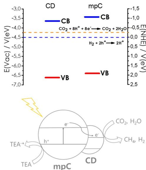
Scheme 2 Band energy diagram and proposed reaction mechanism for the photocatalytic CO<sub>2</sub> reduction in the presence of sacrificial electron donor by CD/mpC.
