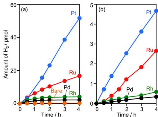
Fig. 1 Sacrificial H<sub>2</sub> evolution from a 10% methanol solution over (a) M (0.05 wt%)/CLTO and (b) Cr<sub>2</sub>O<sub>3</sub>(1.2 wt%)/M(0.05 wt%)/CLTO. Photocatalyst: 0.3 g for (a) and 0.2 g for (b); reactant solution: 10% methanol solution, 160 mL; light source: 300 W Xe lamp ( $\lambda > 420$  nm).
