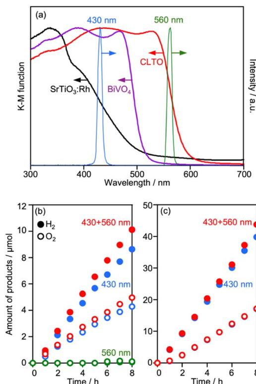
Fig. 10 (a) UV-vis spectra of CLTO, BiVO<sub>4</sub> and SrTiO<sub>3</sub>:Rh reduced by H<sub>2</sub>, and spectra of monochromatic light at 430 and 560 nm. Z-WS in 0.1 mM Co(bpy)<sub>3</sub>SO<sub>4</sub> by (b) Cr<sub>2</sub>O<sub>3</sub>/Ru/CLTO-BiVO<sub>4</sub> and (c) Ru/SrTiO<sub>3</sub>:Rh-BiVO<sub>4</sub> systems under different irradiation conditions.
