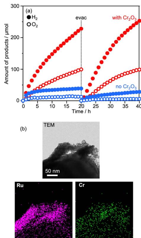
Fig. 9 (a) Influences of  $\text{Cr}_2\text{O}_3$  modification on Z-WS employing  $\text{Ru}(100\% \text{ MeOH})/\text{CLTO}$ . (b) TEM and element mapping images of  $\text{Cr}_2\text{O}_3/\text{Ru}(100\% \text{ MeOH})/\text{CLTO}$ .
