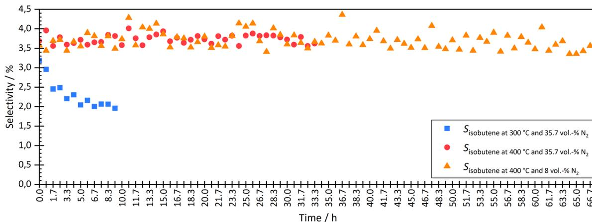
Fig. 5 Comparison the isobutene selectivity over time during coupling at different temperatures (300 °C and 400 °C) and two different  $\text{N}_2$  dilutions (35.7 vol% and 8 vol%).
