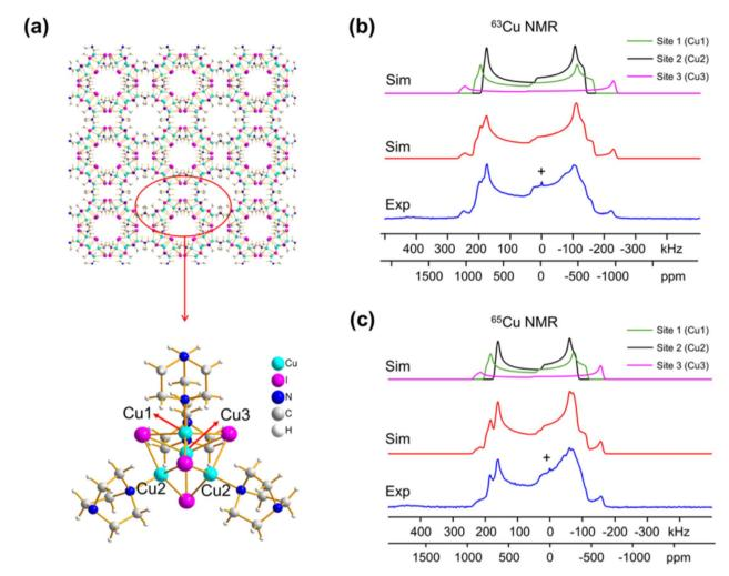
Fig. 1 (a) A schematic diagram of [Cu<sub>4</sub>|<sub>4</sub>(DABCO)<sub>2</sub>] featuring three different Cu sites. The experimental (b) <sup>63</sup>Cu and (c) <sup>65</sup>Cu static NMR spectra (blue), cumulative simulations (red), and individual Cu site simulations (black, purple, green).
