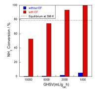
Fig. 2 SV dependence of  $NH_3$  conversion at 398 K over 8.2 mol%  $Ru/CeO_2$ : 300 mg catalyst, 0.1 MPa, and 6.0 mA.
