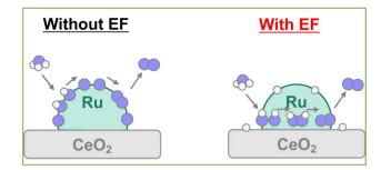
Fig. 9 Schematic image of reaction mechanism under EF.
