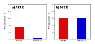
Fig. 1 Temperature dependence of  $NH_3$  decomposition over 8.2 mol%  $Ru/CeO_2$  with and without an electric field: feed, 100%  $NH_3$ , 50 SCCM; catalyst, 100 mg, 0.1 MPa, 0 or 6.0 mA; (a) at 423 K and (b) at 673 K.
