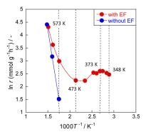
Fig. 3 Arrhenius plots for ammonia decomposition rates over 0.85 mol% Ru/CeO $_2$ : 5% NH $_3$ /Ar = 200 SCCM, 200 mg cat, 0.1 MPa, and 0 or 6.0 mA.
