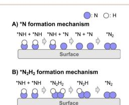
Fig. 4 Schematic image of  $N_2$  formation mechanisms of two types: (A) \*N formation mechanism and (B) \* $N_2H_2$  formation mechanism.
