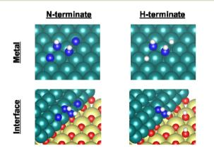
Fig. 5 Catalyst surface models for the respective experiment conditions. Ru, Ce, O, N, and H atoms are shown respectively as green, yellow, red, blue, and white.
