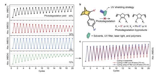
Fig. 3 Photostability of NBDs under two-way photoswitching cycling. (a) Two-way photoswitching cycling test and photodegradation yields of NBDs in MeCN  $(0.1 \text{ mM L}^{-1})$ , where NBD to QC conversion and subsequent QC to NBD back-conversion occur by 365 nm and 265 nm light irradiation, respectively. (b) Scheme of photostability improvement by UV shielding protection. (c) Two-way photoswitching cycling test of NBD4 using solvent and a light filter to cut off deep UV wavelengths.
