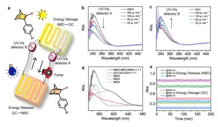
Fig. 5 Two-way photo-switching system in an automated flow device. (a) Automated flow device incorporating the two-way photoswitching MOST system. UV-Vis detectors A and B tested the photoisomerization states after 365 nm and 265 nm light irradiation, respectively. UV-Vis absorption spectra of NBD4 with flow rates in (b) UV-Vis detector A and (c) detector B. (d) UV-Vis absorption spectra of the multi-NBD system. (e) Dynamic photoisomerization processes in the automation flow MOST device.
