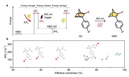
Fig. 4 Energy storage and release under two-way photoswitching cycles. (a) Illustration of a two-way photoswitching MOST system. (b) A comparison of the energy density from the latest reports in two-way photoswitching molecules: O, alkyl azobenzene derivatives;52-56  $\triangle$ , orthofunctionalized azobenzene derivatives;  $^{57}$   $\nabla$ , pyrazole-based azobenzene derivatives;  $^{6,9,58}$   $\stackrel{\star}{\Rightarrow}$ , and this paper.
