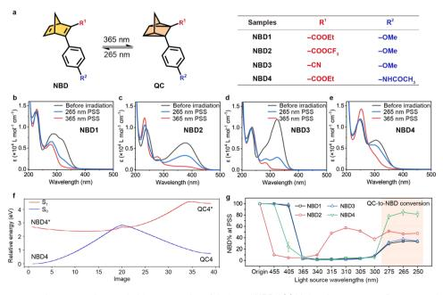
Fig. 1 Molecular structure and two-way photoswitching properties of designed NBDs. (a) Molecular structure of two-way photoswitching NBDs. UV-Vis absorption spectra of (b) NBD1, (c) NBD2, (d) NBD3, and (e) NBD4 in an MeCN solution (0.1 mM  $L^{-1}$ ). (f) Photoisomerization paths between NBD4 and QC4 *via* the minimum energy conical intersection. (g) Photoisomerization yields using 11 different irradiation wavelengths of NBDs at photostationary states (PSSs) in a MeCN solution.
