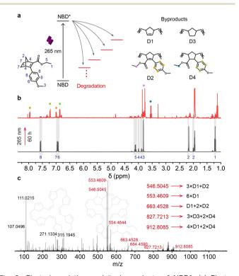
Fig. 2 Photodegradation and its byproducts of NBD1. (a) Photodegradation mechanism NBD1 under 265 nm light irradiation. (b)  $^1\mathrm{H}$  NMR spectra and of NBD1 before and after 265 nm light irradiation. (c) HRMS spectrum of NBD1 after 265 nm light irradiation.
