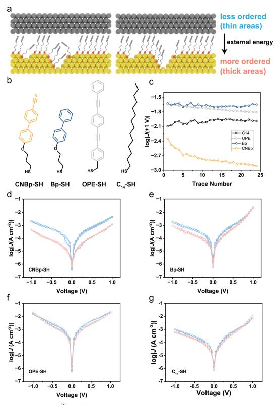
Fig. 1 (a) Schematic illustration of  $Au^{TS}$ -SAM// $Ga_2O_3$ /EGaIn molecular junctions. (b) Chemical structures of the thiol precursors. (c) Plots of tunneling current  $\log |J(+1.0 \text{ V})|$  versus sweep number for the molecular junctions. (d-g)  $\log |J(V)|$  plots for the molecular junctions at the first sweep and last sweep.
