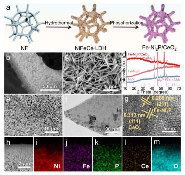
Fig. 1 (a) Schematic illustration of the preparation process for Fe-Ni<sub>2</sub>P/CeO<sub>2</sub>. (b and c) SEM images of NiFeCe LDH. (d) XRD patterns of Ni<sub>2</sub>P, Fe-Ni<sub>2</sub>P and Fe-Ni<sub>2</sub>P/CeO<sub>2</sub>. (e) SEM, (f) TEM, (g) HRTEM, (h-m) SEM and corresponding element mapping images for Fe-Ni<sub>2</sub>P/CeO<sub>2</sub>.
