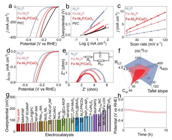
Fig. 3 (a) Polarization curves and (b) Tafel slopes for Ni<sub>2</sub>P, Fe-Ni<sub>2</sub>P/CeO<sub>2</sub> and Pt/C. (c) C<sub>dl</sub> values, (d) ECSA-normalized polarization curves, (e) EIS and (f) HER performance radar chart for Ni<sub>2</sub>P, Fe-Ni<sub>2</sub>P and Fe-Ni<sub>2</sub>P/CeO<sub>2</sub>. (g) Comparison of HER performances of Fe-Ni<sub>2</sub>P/CeO<sub>2</sub> with the developed catalysts. (h) Stability test for Fe-Ni<sub>2</sub>P/CeO<sub>2</sub>
