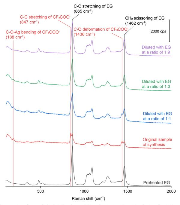
Fig. 4 Raman spectrum of preheated EG and SERS spectra recorded from the original reaction solution of Ag irregular particles synthesized using  $CF_3COOAg$  and after it had been diluted with the EG at various ratios.
