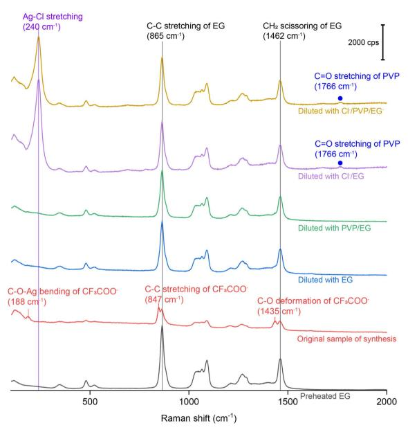
Fig. 3 Raman spectrum of the preheated EG, SERS spectra of the as-obtained Ag irregular particles in the original reaction solution containing no  $Cl^-$  and after it had been diluted by 10 times with EG, EG containing PVP, EG containing  $Cl^-$ , and EG containing both PVP and  $Cl^-$ .
