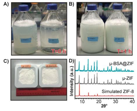
Fig. 7 Scaled synthesis of  $\mu$ -ZIF and  $\mu$ -BSA[Cy7]@ZIF. (A) Image of 2 L bottles (left:  $\mu$ -BSA@ZIF, right:  $\mu$ -ZIF) used for scaled-up ZIF synthesis at T= 0 h and (B) at T = 1 h. (C) 15.9 q of  $\mu$ -ZIF powder (left) and 16.4 q  $\mu$ -BSA[Cy7]@ZIF powder (right) from 2 L synthesis. (D) PXRD diffractograms of  $\mu$ -BSA[Cy7]@ZIF (top),  $\mu$ -ZIF (middle), and simulated ZIF-8 (bottom) following scaled synthesis.
