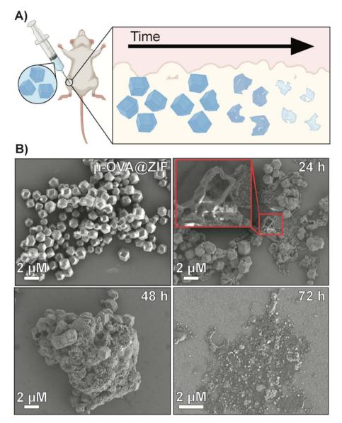
Fig. 4 Degradation analysis of  $\mu$ -OVA@ZIF post-injection. (A) Schematic representation of the degradation of ZIF-8 crystals *in vivo*. (B) SEM images of pristine  $\mu$ -OVA@ZIF and the *ex vivo* extracts at 24 h, 48 h, and 72 h post-injection.
