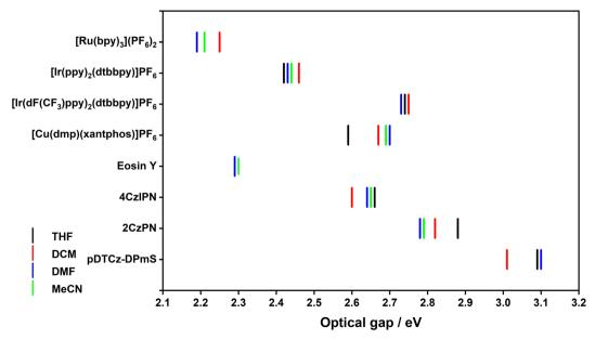
Fig. 6 Variation of optical gap with solvent for the eight PCs.
