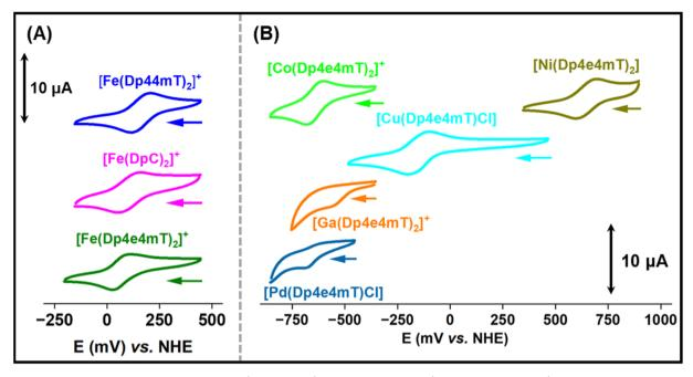
Fig. 4 Cyclic voltammograms of: (A)  $[Fe(Dp44mT)_2]^+$ ,  $[Fe(DpC)_2]^+$ , and  $[Fe(Dp4e4mT)_2]^+$ . (B)  $[Co(Dp4e4mT)_2]^+$ ,  $[Ni(Dp4e4mT)_2]^+$ ,  $[Ni(Dp4e4mT)_2]^+$ ,  $[Ni(Dp4e4mT)_2]^+$ , and [Pd(Dp4e4mT)Cl] (1 mM in MeCN/H<sub>2</sub>O 7:3 (v/v) + 0.1 M Et<sub>4</sub>NClO<sub>4</sub>) at a sweep rate of 100 mV s<sup>-1</sup>. The voltammograms were recorded using a glassy carbon working electrode *versus* a non-hydrogen electrode (NHE).
