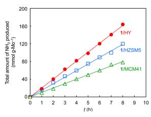
Fig. 2 Catalytic performance of ammonia synthesis at 400 °C and 1.0 MPa (absolute pressure) using (H<sub>3</sub>O)<sub>2</sub>[(Mo<sub>6</sub>Cl<sub>8</sub>)Cl<sub>6</sub>]·6H<sub>2</sub>O (1)/HY,  $(H_3O)_2[(Mo_6Cl_8)Cl_6] \cdot 6H_2O$  (1)/HZSM5, and  $(H_3O)_2[(Mo_6Cl_8)Cl_6] \cdot 6H_2O$ (1)/MCM41 as precursors. Catalyst amount, 0.2 g; N<sub>2</sub>/H<sub>2</sub> (1/3-mixture) flow rate, 60 mL min<sup>-1</sup>.
