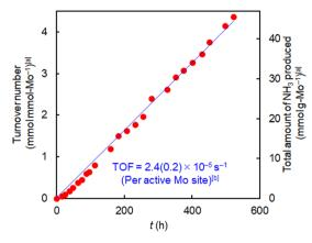
Fig. 3 Ammonia synthesis using  $(H_3O)_2[(MO_6Cl_8)Cl_6] \cdot 6H_2O$  (1)/HY at 200 °C and 5.0 MPa (absolute pressure). Catalyst amount, 0.2 g;  $N_2/H_2$  (1/3-mixture) flow rate, 60 mL min<sup>-1</sup>. [a] Per Mo included in the catalysts. [b] Per NH<sub>3</sub>-adsorbing Mo (see Table S4†).
