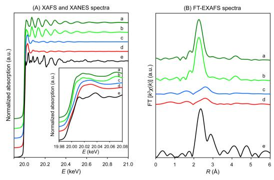
Fig. 1 (A) XAFS spectra of (H<sub>3</sub>O)<sub>2</sub>[(Mo<sub>6</sub>Cl<sub>8</sub>)Cl<sub>6</sub>]·6H<sub>2</sub>O (1). The inset shows the XANES region. (B) FT-EXAFS spectra of 1: (a) as prepared, (b) 1/HY after impregnation, (c) 1/HY after H<sub>2</sub>-activation, and (d) 1/HY after NH<sub>3</sub>-synthesis. Spectrum of Mo foil from the Spring-8 BENTEN database (https://doi.org/10.48505/nims.2249) (e) is also shown.
