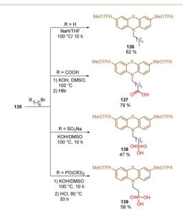
Scheme 17 Synthesis of phenothiazines with different anchoring groups: -H 136, -COOH 137, -SO<sub>3</sub>H 138, and -PO(OH)<sub>2</sub> 139.
