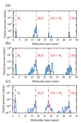
Fig. 8 Mass spectral analysis of the gas species that are present in the UHVDS: (a) "empty" system; (b) a pre-treated PA2200 nylon segment of L = 50 mm fabricated by the SLS EOS Formiga P100 3D printer, and (c) a pre-treated high-temperature resin channel of L = 500 mm fabricated by the SLA Formlabs Form 3 3D printer inserted inside the diffusion channel. The analysis is conducted using the SRS RGA100 mass spectrometer.
