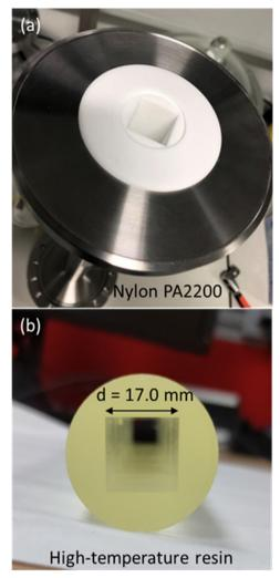
Fig. 9 Photographs of two channels with a square cross section with edge length of 17 mm and channel length of 500 mm, made of: (a) PA2200 nylon using an SLS EOS Formiga P100 3D printer, and (b) high-temperature resin using an SLA Formlabs Form 3 3D printer.
