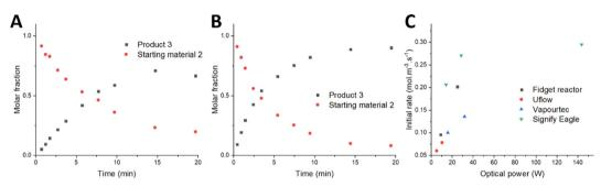
Fig. 6 A) Evolution of the reaction composition (molar fraction based on reagent 2 and product 3) at different reaction times in the Uflow reactor. B) Evolution of the reaction composition (molar fraction based on reagent 2 and product 3) at different reaction times in the Fidget reactor, C) Initial rate of the chemical transformation at different optical power for the different reactor designs.
