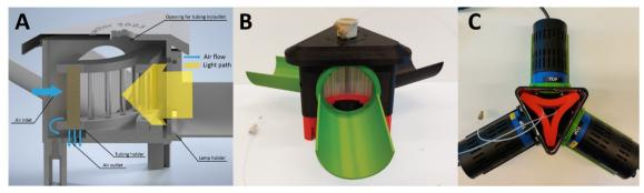
Fig. 3 A) Sliced schematic design of the Fidget reactor system with air flow and light path directions indicated. B) Assembled reactor system built and ready for operation, showing the wound capillary in its custom holder. C) Top view of the opened Fidget reactor equipped with the 3 Kessil lamps.
