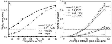
Fig. 5 Larger grains induce internal diffusion limitations. (A) Weisz-modulus of 2.6\_Pd/C (solid line, filled symbols) and 0.01\_Pd/C (dashed line, open symbols) catalysts with average catalyst grain size of 19 µm (circles) or 180 µm (triangles). (B) Overview of the Weisz-moduli for the tested combinations of Pd loading and grain size at lowest (25 °C) and highest (100 °C) tested temperature.
