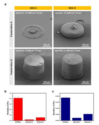
Fig. 2 (a) Effect of SOG (0.02 wt%) as a resolution enhancer and fumed silica (15 wt%) as an anti-sticking agent, as SEM images of 3Dprinted cylinders. (b) Modulus and (c) hardness of 3D-printed PMMA, hybrid 2, and hybrid 4.
