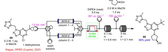
Scheme 25 Telescoped amine scavenging with nucleophilic aromatic substitution in flow using in-line UV-vis spectrometry developed by Kappe and co-workers.<sup>67,68</sup>
