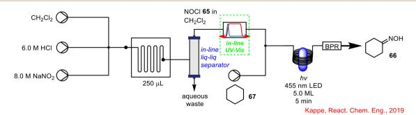
Scheme 24 Telescoped NOCI 65 generation with photochemical synthesis of cyclohexanone oxime 66 using in-line UV-vis spectrometry to monitor NOCl 65 concentration.64
