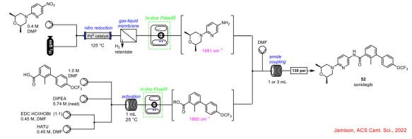
Scheme 19 Schematic of flow synthesis of sonidegib 52 (ref. 58).
