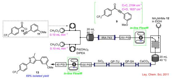
Scheme 4 FlowIR to enhance production and safety of telescoped process by Ley and co-workers.<sup>37</sup>
