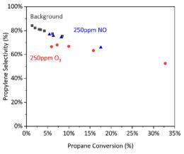
Fig. 8 Selectivity vs. conversion for radical-activated gas-phase reactions. Conditions: 490 °C, 30%  $C_3H_8/{\sim}15\%$   $O_2/{\sim}55\%$   $N_2$ , 67–200  $L_{C_zH_o}^N$   $L^{-1}$   $h^{-1}$ , 9 mm ID tube section.
