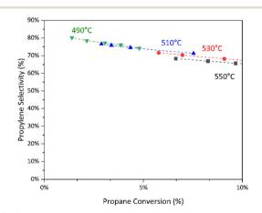
Fig. 4 Propylene selectivity vs. propane conversion over boron nitride at various temperatures. Conditions: 490-550 °C, 30% C<sub>3</sub>H<sub>8</sub>/15% O<sub>2</sub>/ 55%  $N_2$ , 100 mg hBN diluted in 500 mg passivated SiC, 29–94  $g_{C_3H_8}$  $g_{hBN}^{-1} h^{-1}$ , 7 mm ID tube.
