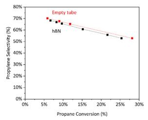
Fig. 1 Selectivity to propylene vs. conversion for hBN and empty tube. Conditions: 550 °C, 30%  $C_3H_8/15\%$   $O_2/55\%$   $N_2$ , 680–2200  $L_{C_3H_8}^N$   $L^{-1}$   $h^{-1}$  (hBN) or 100–200  $L_{C_3H_8}^N$   $L^{-1}$   $h^{-1}$  (empty tube).
