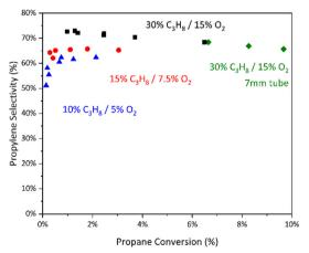
Fig. 3 Propylene selectivity vs. propane conversion over boron nitride at various feed dilutions. Each run maintained a 2:1 C3H8: O2 ratio but with a different feed dilution to achieve the stated feed fraction of C<sub>3</sub>H<sub>8</sub>. Conditions: 550 °C, 20-80 mLn min<sup>-1</sup>, 1:5 dilution of boron nitride in passivated silicon carbide (50 mg hBN in 4 mm tube and 100 mg hBN in 7 mm tube). All runs were performed in a 4 mm tube unless otherwise noted
