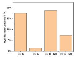
Fig. 2 Comparison of conversion of C<sub>3</sub>H<sub>8</sub> and C<sub>3</sub>H<sub>6</sub> over hBN in the presence/absence of NO. Conditions: 550 °C, 7 mm tube, ~30% C<sub>3</sub>H<sub>8</sub> or  $C_3H_6/15\%$   $O_2/0$  or 150 ppm  $NO/\sim55\%$   $N_2$ , 40 mLn min<sup>-1</sup> total flow, 100 mg hBN diluted in 500 mg SiC.
