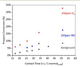
Fig. 7 Light-off of propane conversion from the introduction of O<sub>3</sub> or NO. Conditions: 490 °C, 30%  $C_3H_8/{\sim}15\%$   $O_2/{\sim}55\%$   $N_2$ , 67–200  $L_{C_3H_8}^N$  $L^{-1} h^{-1}$ , 9 mm ID tube section.
