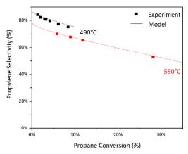
Fig. 5 Microkinetic model prediction vs. experimental observations for gas-phase selectivity vs. conversion at 490 °C and 550 °C. Conditions: 490-550 °C, 30% C<sub>3</sub>H<sub>8</sub>/15% O<sub>2</sub>/55% N<sub>2</sub>, 67-200 L<sup>N</sup><sub>C<sub>2</sub>H<sub>0</sub></sub> L<sup>-1</sup> h<sup>-1</sup>, 9 mm ID tube.
