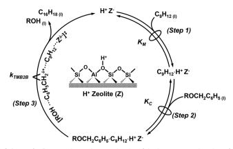
Scheme 2 Proposed reaction mechanism (via the concerted pathway) for benzylation of mesitylene (C9H12) with a benzylating agent  $(ROCH_2C_6H_5)$  on a Brønsted acid site  $(H^+Z^-)$  to form 1,3,5-trimethyl-2benzylbenzene (C<sub>16</sub>H<sub>18</sub>) and a leaving group (ROH). Steps are described in the text.
