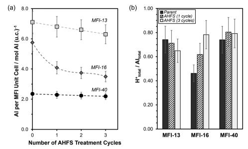
Fig. 2 (a) Total Al content per MFI unit cell (96 T atoms) and (b) bulk H<sup>+</sup>tot/Altot molar ratio as a function of the number of AHFS-treatment cycles. Dashed lines in (a) serve to guide the eye. Error bars in (a) reflect uncertainties (±10% in (a) and ±15% in (b)).
