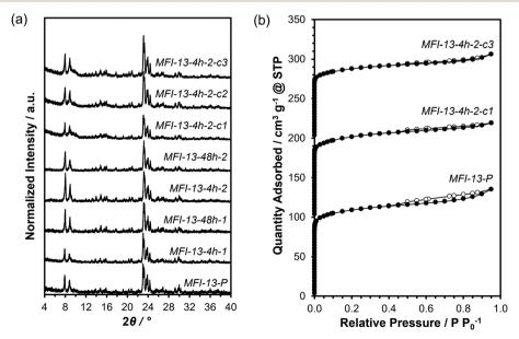
Fig. 1 (a) Powder XRD patterns and (b) N2 adsorption (closed)-desorption (open) isotherms (77 K) of parent MFI-13 (MFI-13-P) and AHFS-treated MFI-13 (MFI-Si/Al-duration-concentration-cycle#). The isotherms were vertically offset by 100 cm $^3$  g $^{-1}$  for clarity.
