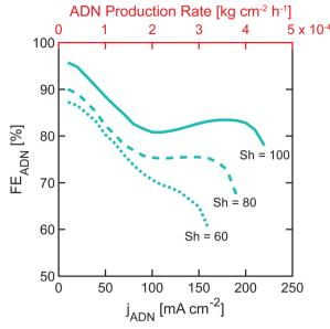
Fig. 8 Unified model GPR predicted Pareto fronts showing the performance tradeoffs between ADN faradaic efficiency (FE<sub>ADN</sub>) and ADN partial current density  $(j_{ADN})$  for several convection conditions. The ADN production rate (top axis - red) is directly proportional to  $i_{ADN}$ . Pareto fronts for three Sherwood numbers (Sh = 60, 80, 100) are shown
