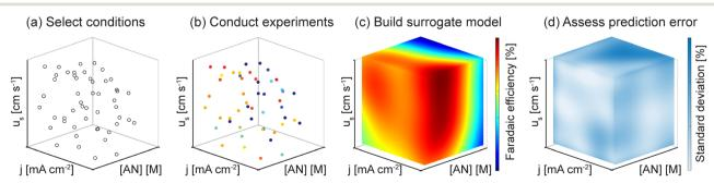
Fig. 3 Illustration of the process for building data-driven surrogate models. (a) Pseudorandom experimental conditions are selected using Latin hypercube sampling (LHS), (b) experimental data is collected by performing electrochemical reactions at the selected conditions, (c) surrogate models are built using Gaussian process regression (GPR), and (d) standard deviations of the predictions are assessed.
