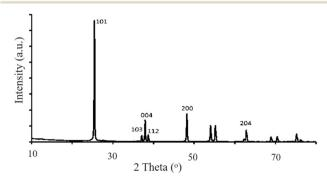
Fig. 3 XRD pattern of the TiO<sub>2</sub> powder.
