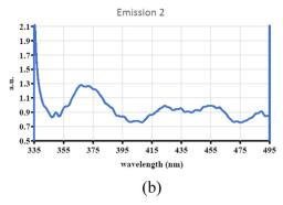
Fig. 1 Solid-state spectra for the anatase powder. (a) Electronic absorption spectra measured for a suspension of 0.1 q TiO<sub>2</sub> in 50 mL water, and (b) photoluminescence spectra measured for the solid TiO<sub>2</sub> film under 300 nm excitation wavelength. All measurements were carried out at room temperature.
