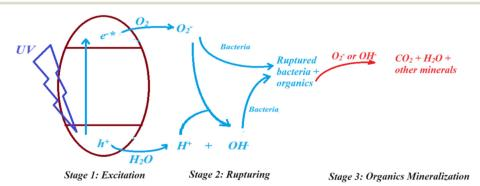
Fig. 7 Schematic showing a mechanism summary proposed for TiO<sub>2</sub> nanoparticles as a catalyst for the photo-degradation of aqueous bacteria, followed by their organic components. All stages are based on earlier literature.
