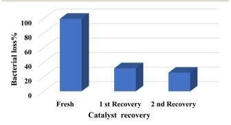
Fig. 6 Effect of powder catalyst recovery and reuse on *S. aureus* loss. Experiment conducted using fresh anatase TiO<sub>2</sub> (0.1 g), first recovered and second recovered catalyst. Fresh bacterial solution (50 mL,  $1\times10^6$  CFU mL<sup>-1</sup>) is used in each catalyst, with pH 6.2, for 1 h at 25  $\pm$  2 °C under a radiation intensity of 0.136 W cm<sup>-2</sup>. Error is 10%.
