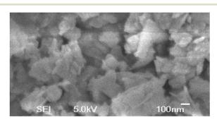
Fig. 2 SEM image of the solid commercial anatase TiO<sub>2</sub> powder.
