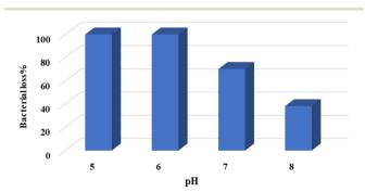
Fig. 5 Effect of pH value on S. aureus bacterial loss. Experiments conducted using 0.1 g TiO<sub>2</sub> powder, and 1 × 10<sup>6</sup> CFU mL<sup>-1</sup> in 50 mL bacterial mixture at 25  $\pm$  2  $^{\circ}$ C under a radiation intensity of 0.136 W cm<sup>-2</sup>. Error is 10%.
