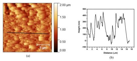
Fig. 4 AFM image of the TiO<sub>2</sub> film deposited on a glass surface: (a) surface analysis, and (b) height profiling
