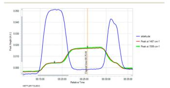
Fig. 2 Consumption of aldehyde starting material when hydrazine reagent is injected, and identification of peaks at 1487 cm<sup>-1</sup> and 1599 cm<sup>-1</sup> indicative of the presence of the intermediate.
