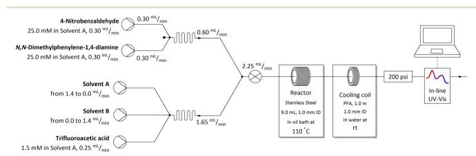
Fig. 5 Flow setup and reaction conditions used in solvents mixtures studies in imine formation reaction.
