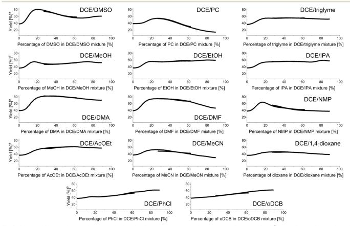
Fig. 6 Results of binary solvents mixtures studies in imine formation reaction under continuous flow conditions. <sup>a</sup>Yield at fixed residence time of 240 seconds
