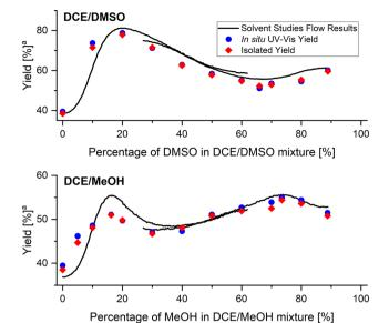
Fig. 7 Comparison of flow and validation results of imine formation reaction. a Yield at fixed residence time of 240 seconds.
