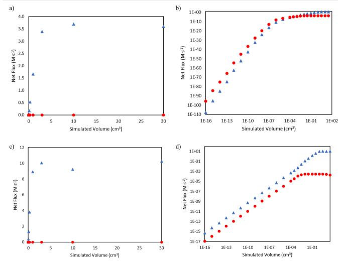
Fig. 6 Comparisons of net flux of nonenyl  $\beta$ -scission (blue triangles  $\triangle$ ) and nonyl  $\beta$ -scission (red circles  $\bigcirc$ ) as a function of reactor volume. a) Total pressure 15 bar, linear scale b) total pressure 15 bar, log-log scale c) total pressure 25 bar, linear scale d) total pressure 25 bar, log-log scale.
