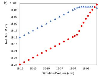
Fig. 5 Comparison of rates of hydrogen abstraction from ethylene by 1,4-butyl diradical (blue triangles ) and butene diradical (red circles as a function of reactor volume. a) Total pressure 15 bar b) total pressure 25 bar.
