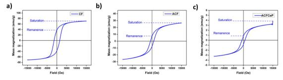
Fig. 7 Magnetic hysteresis (M-H) curve of cobalt ferrite (CF) (a); Ag-doped cobalt ferrite (ACF) (b) and ACFCeP composite (c).
