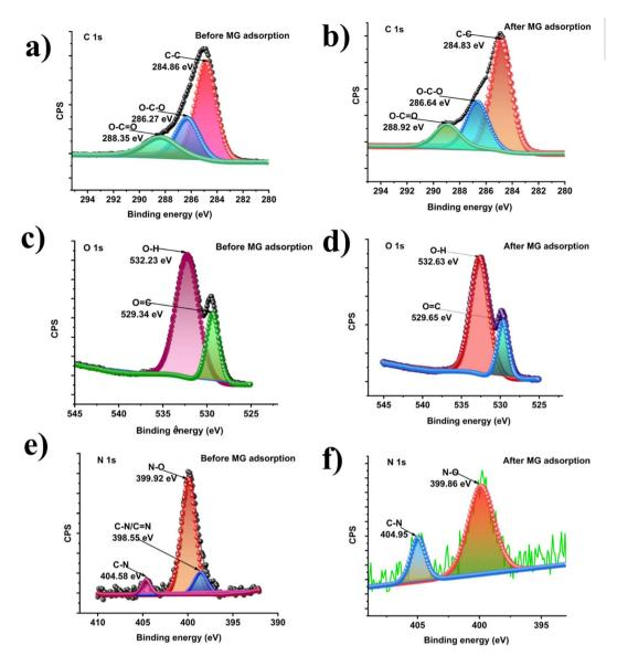
Fig. 3 XPS deconvoluted C 1s spectra of the ACFCeP composite before adsorption (a) and after adsorption (b); O 1s spectra of the ACFCeP composite before adsorption (c) and after adsorption (d); N 1s spectra of the ACFCeP composite before adsorption (e) and after adsorption (f).
