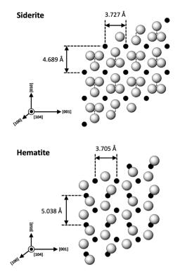
Fig. 15 Projection of the atomic structures of a (104) slices of hematite and siderite showing the main directions of epitaxy and repeating periods.
