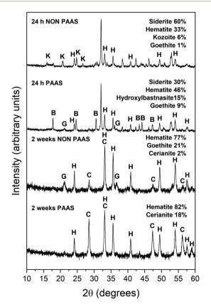
Fig. 2 Powder XRD patterns of goethite (G), hematite (H), kozoite (K), hydroxylbastnasite (B) and cerianite (C) in the equal concentration (non-PAAS) and PAAS experiments at 165 °C after 24 hours and 2 weeks (Bragg peaks that have not been assigned to any phase correspond to siderite).
