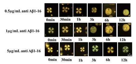
Fig. 5 Polarized optical microscope images of LC droplets of different concentrations of antibody (anti A $\beta$ 1-16) at particular concentration antigen A $\beta$ 1-42 at 67.5  $\mu$ M.
