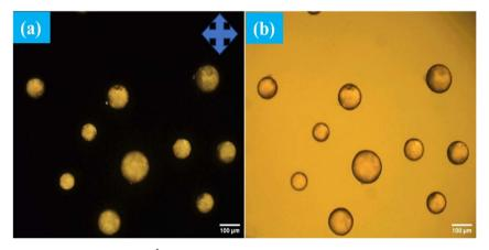
Fig. 8 POM images of immobilized antibody 1  $\mu$ g mL<sup>-1</sup> on surfaces of LC droplets at pH 7.4 after addition A $\beta$ 1–42 at concentration of 112.5  $\mu$ M with (a) and without (b) cross polarizer.
