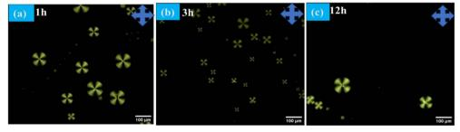
Fig. 4 Polarizing optical microscope images of LC microdroplets anchoring with anti A $\beta$ 1-16 with different incubation times (a) 1 h (b) 3 h (c) 12 h at 10  $\mu$ g mL<sup>-1</sup> concentration.
