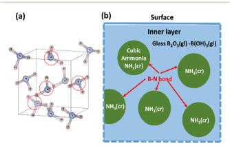
Fig. 1 (a) Unit cell of cubic  $NH_3(cr)^{24-26}$  composed of four molecules marked with open circle; (b) schematic model for stabilising the solid-state cubic ammonia ( $NH_3(cr)$ ) at ambient temperature, which is otherwise only stable below 195.5 K under atmospheric pressure.
