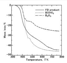
Fig. 8 TG analyses of the samples prepared from freeze-drying (FD product), commercial  $B(OH)_3(cr)$  and  $B_2O_3(cr)$ , respectively. The initial masses of FD product, commercial  $B(OH)_3(cr)$  and  $B_2O_3(cr)$  were 19.2, 20.6 and 13.7 mg, respectively.
