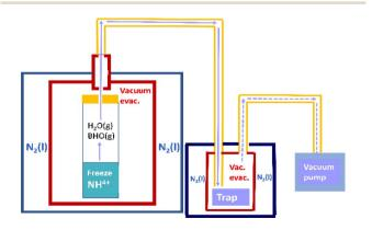
Fig. 2 Schematic of freeze-drying apparatus and method for synthesising the solid-state cubic-NH<sub>3</sub>(cr).
