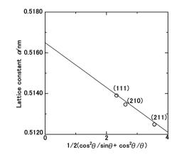
Fig. 5 Lattice constant as function of the diffraction degree,  $\theta$ , for the solid-state cubic ammonia (NH $_{3}$ (cr)) at 297 K.
