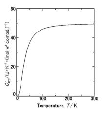
Fig. 7  $C_{p,m}^{\circ}$  data from thermodynamic simulation for solid state cubic NH<sub>3</sub>(cr) (Table S2†).
