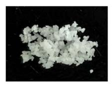
Fig. 3 FD product obtained through freeze-drying, comprising solid-state cubic  $NH_3(cr)$  as the main constituent.
