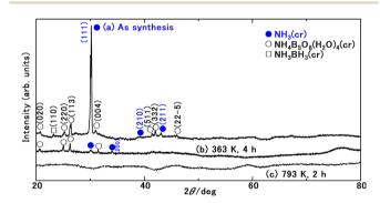
Fig. 4 XRD patterns of reaction products comprising the solid-state cubic ammonia (NH $_3$ (cr)) as main product, ammonium pentaborate (NH $_4$ B $_5$ O $_8\cdot$ 4H $_2$ O(cr)) (open circle), and ammonia borane (NH $_3$ BH $_3$ (cr)) (open square) as the sub-products.
