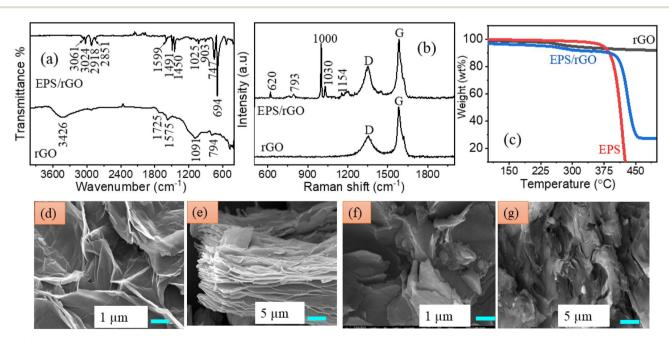
Fig. 2 (a) FT-IR (b) Raman spectrum of pure rGO and EPS/rGO composite (c) TGA curves of rGO, EPS, EPS/rGO (d, e) FE-SEM images pure rGO (f, g) FE-SEM images of EPS/rGO composite.
