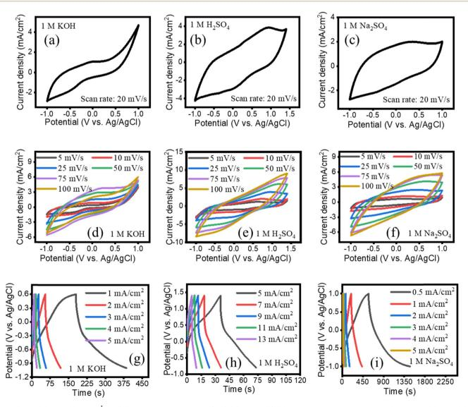
Fig. 5 (a, b, c) CVs at 20 mV s<sup>-1</sup> (d-f) CVs at various scan rates (g-i) GCD of EPS/rGO composite recorded in 1 M KOH, 1 M  $H_2SO_4$ ,  $Na_2SO_4$  aqueous electrolyte.
