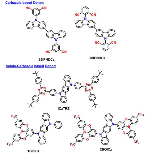
Fig. 2 Chemical structures of A-D-A type TADF materials based on carbazole and indolocarbazole based donors.
