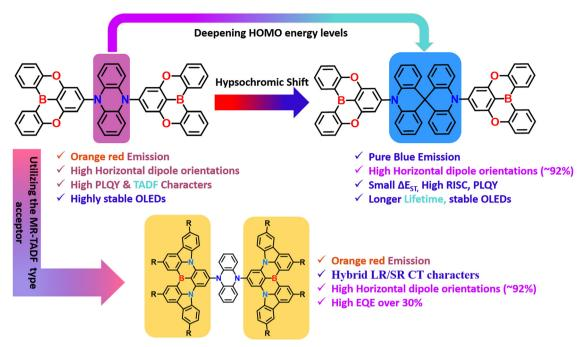
Fig. 5 Comparison of the effect of donor and acceptors in boron based A-D-A type TADF emitters
