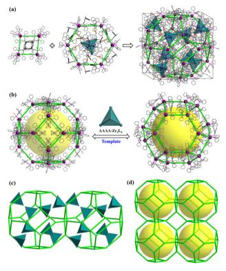
Fig. 2 Packing structure of PTC-374(S,Λ): (a and b) formation of  $\Lambda\Lambda\Lambda\Lambda$ -Zr<sub>4</sub>L<sub>6</sub> cage-supported zeolite SOD-type supramolecular framework and its simplified topology network (c and d).
