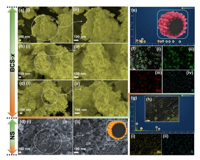
Fig. 2 FE-SEM images of the (a) BCS-0.5, (b) BCS-1, (c) BCS-2, and (d) NS materials at different magnifications. (e) and (g) EDS spectra and (f) (i)—(iv) and (h) (i), (ii) elemental mapping images of the BCS-1 and NS materials, respectively.
